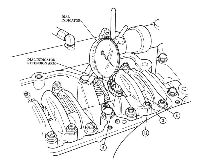
13. Loosen locknut (1) on intake rocker lever (3) of cylinder No. 5 and back out adjusting screw (2).
